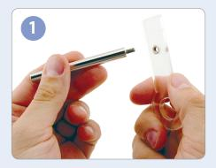
Choose a mandrel based on the desired jump ring size; screw it into the base.
