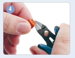
Once the wire is coiled, remove it from the base and cut with a Beadalon Flush Cutter.
